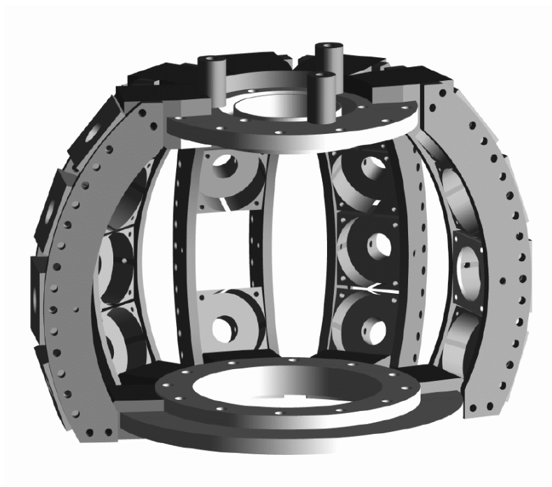
Figure 5.16: Drawing of the Silicon Ball charged-particle detector in the configuration as used in the experiment. The silicon detectors themselves are not shown. One position is left open for the beam to pass through.
