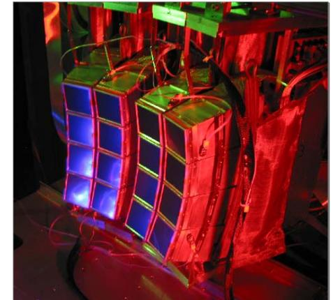
HiRA is an array of charged particle detectors:
