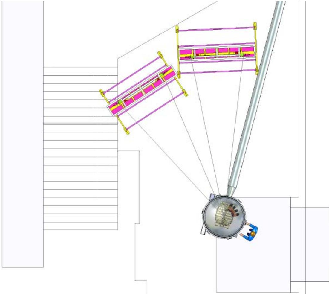
Figure 5: Overhead view of setup in the reconfigured S2 vault involving Miniball, LASSA (at forward angles) and two neutron walls.
