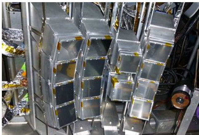
Fig. 10. The High Resolution Array (HiRA). In this picture, HiRA is arranged at forward angles for a transfer reaction measurement.
