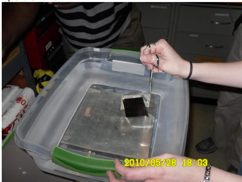
Figure 8. Approach the carbon foil with the frame fully submerged. Align the edge of the foil with the top of the frame.
